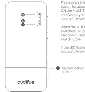
Please press the multi-function button for about 3 seconds to switch ON the MULTISTREAMER PRO. If the LED flashes green 5 times, you have successfully switched ON your device.
