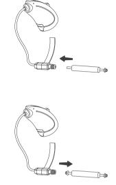
First remove the dome from the receiver module and clean it.
